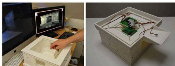
Fig. 7: Virtex uses a low-cost 3d print of an object to embed sensors. Visitors can have a direct feedback by touching the surface (Ara Pacis). (Courtesy of Visual Dimension)
