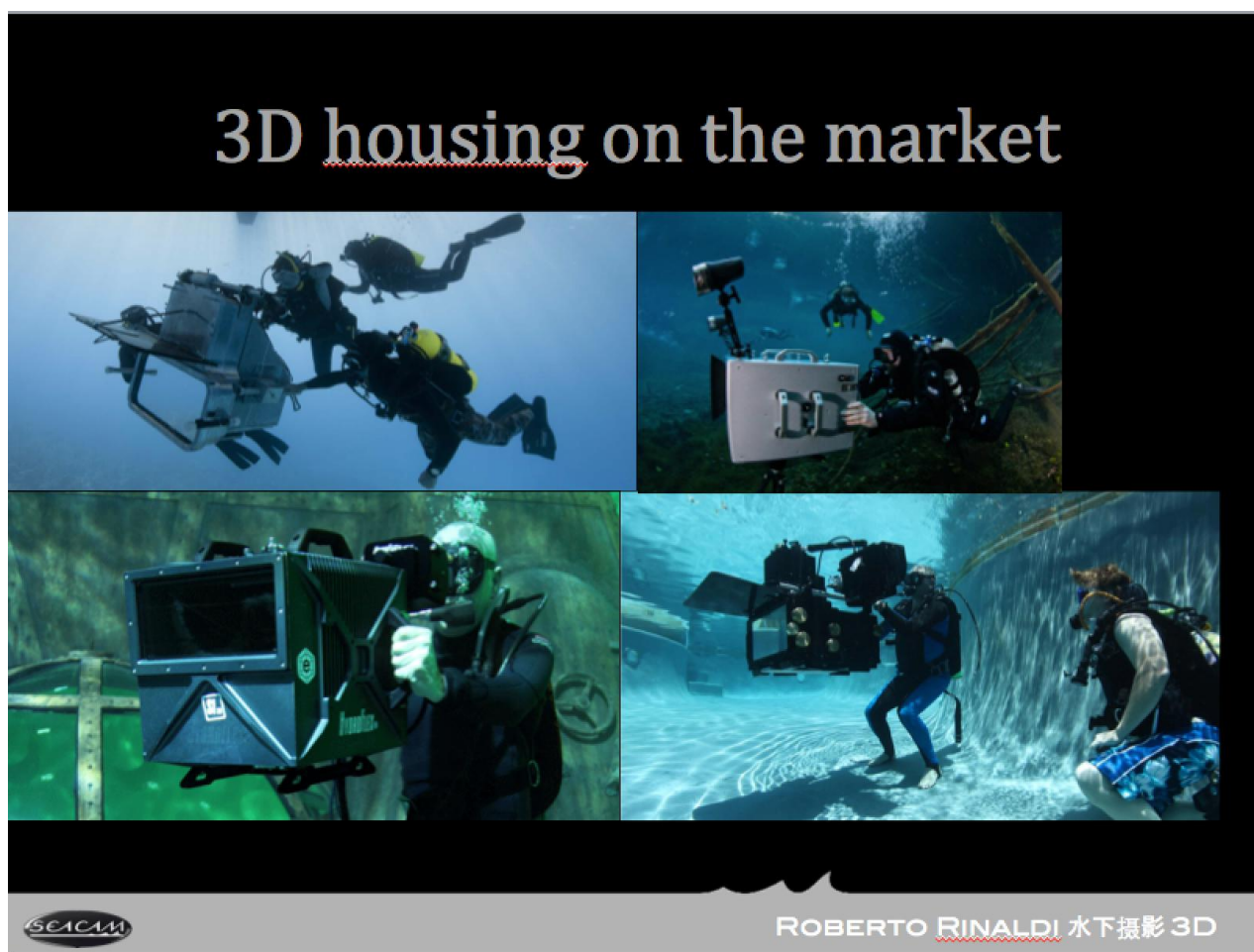
Fig. 1: Some of these housings have been used for successful movies. But almost all in a controlled environment and with a lot of constrains. The large size and the very wide flat port are evident. Furthermore, the reflection of the camera on the flat port may be also very important: imposing the use of very big shader that hinders underwater movement.
