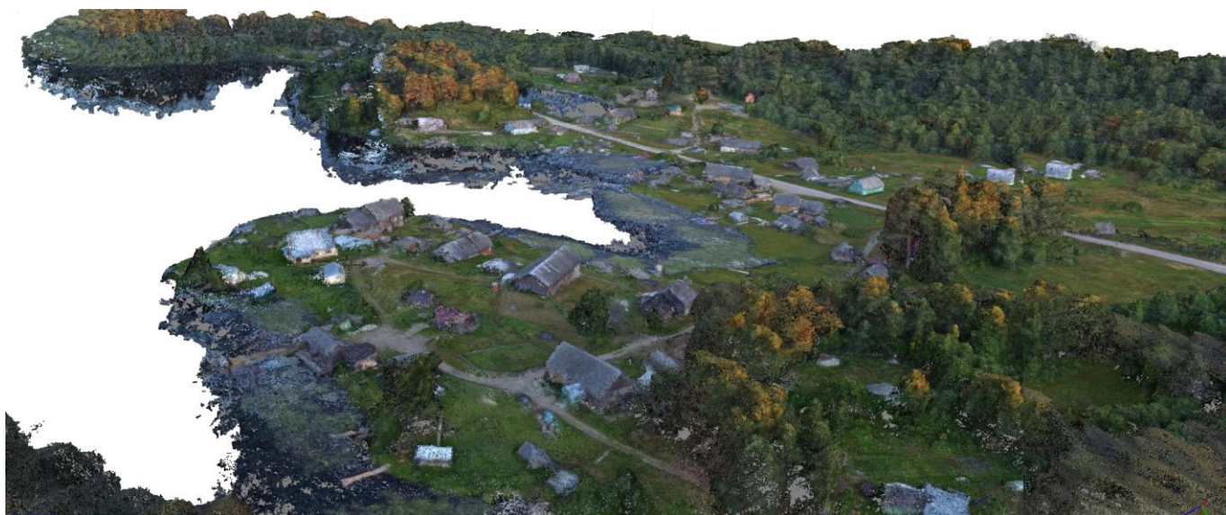
Fig 7: 3D model of the village of Sierghilachta. The photographic campaign was carried out at high altitude using a motorised hang glider. Using this it was possible to fly over the whole village and take photographs from various viewpoints to cover the entire area. The uniform exposure of the various fronts and absence of clear-cut shadows made for a model without omissions, providing a valid basis for studies related to understanding the morphology of the landscape.
