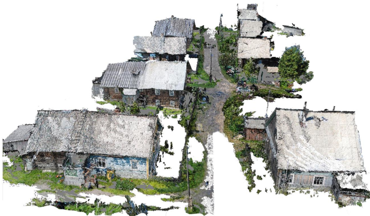
Fig 18: Zenith view of the 3D model. The individual buildings have been joined to the 3D model using reference markers, identifying at least 4 common points between each pair of models.
