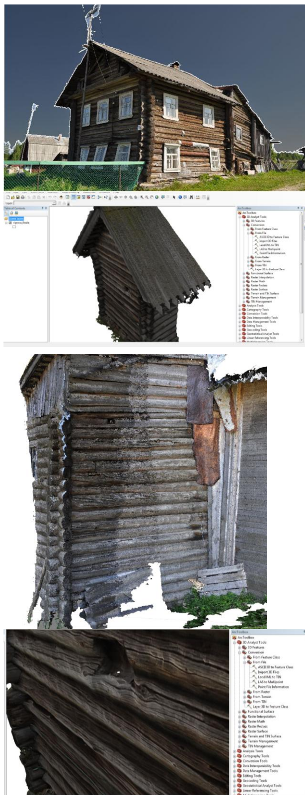
Fig 17: ArcGIS software screens for the creation of 3D GIS databases. The models obtained, appropriately reduced in the number of polygons and optimized in the mesh, can be used and interrogated, integrated by whole range of information that in an instant can provide valuable support to the operations of the documentation of the actual architecture condition.
