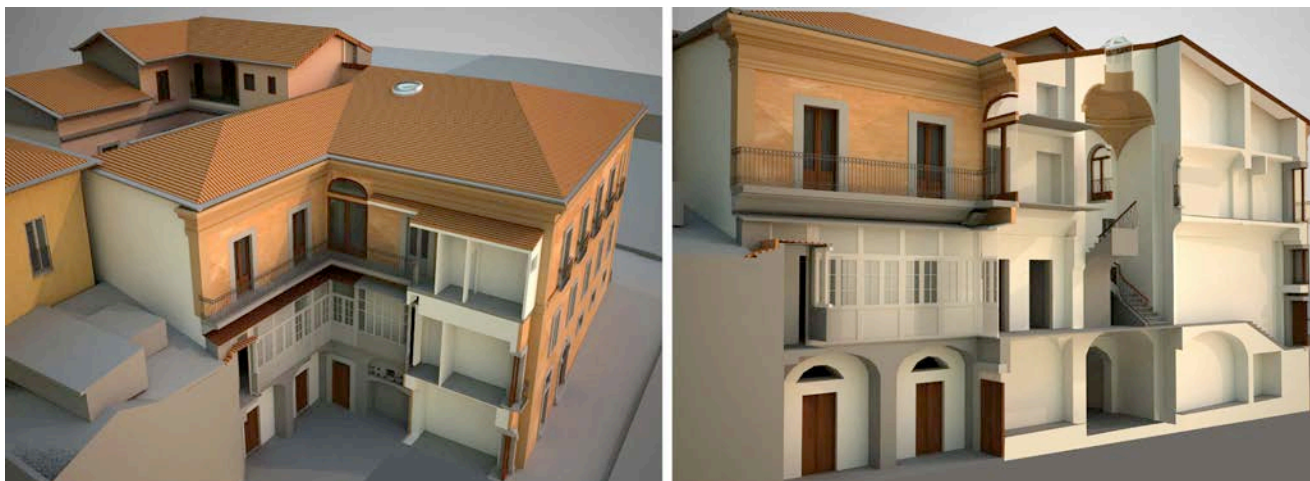
Fig. 10: 3D model of a block of the historical centre. Its articulation is useful for the study of architectural values, of the inside and outside spaces, of building's typologies (F. Cerasoli).
