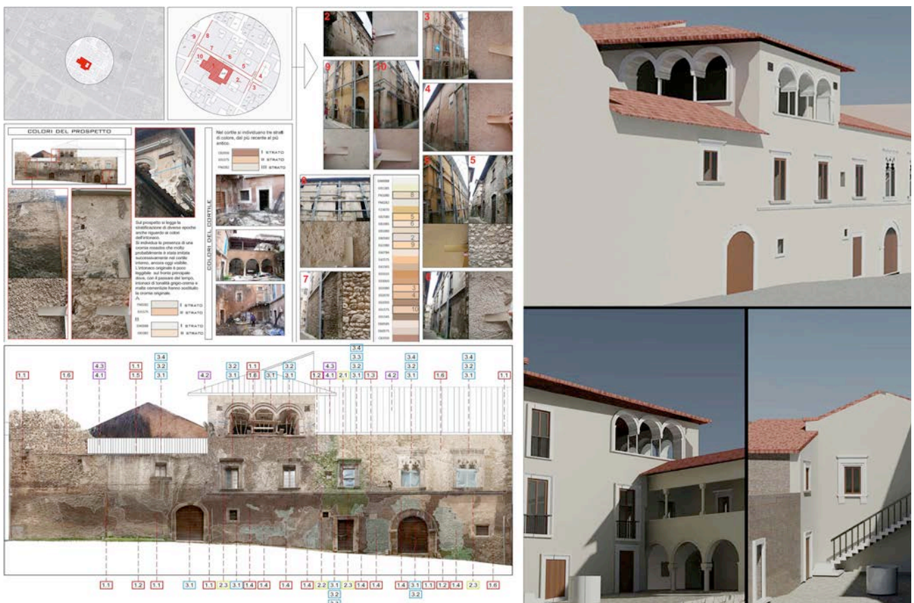
Fig. 5: Study of an urban block’s facade: architectural and constructive elements, materials, colors, and degradation. The 3D model favors the analysis and visualization of the architectural characteristics. (A. Gaeta, M. Mattei, P. Pifano, F. Tresca – Prof. M. Centofanti, Assistant S. Brusaporci).
