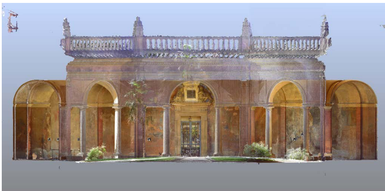
Fig. 7: San Michele in Bosco (Bologna), point cloud of the Carracci cloister.
