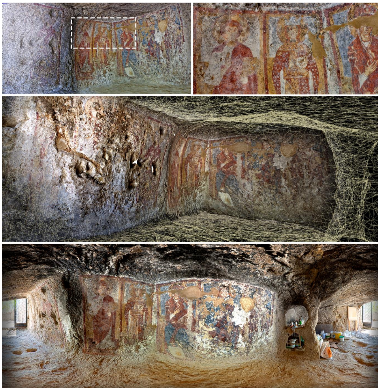
Fig. 4: The Grotto of Saints in Enna - the frescoes. The 3D texture made by photogrammetric techniques (above), the model from 3D laser scanning survey (center), HDR panoramic image made by techniques of photo-stitching (bottom).
