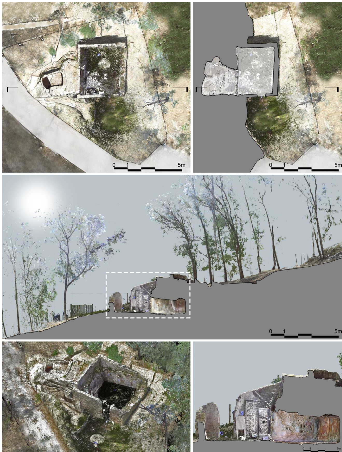
Fig. 3: The Grotto of Saints in Enna - 3D laser scanning, orthographic projections of the point cloud. The planimetry and the floor plan of the cave (above), the longitudinal section (center), the isometric view and details of the interior (bottom).
