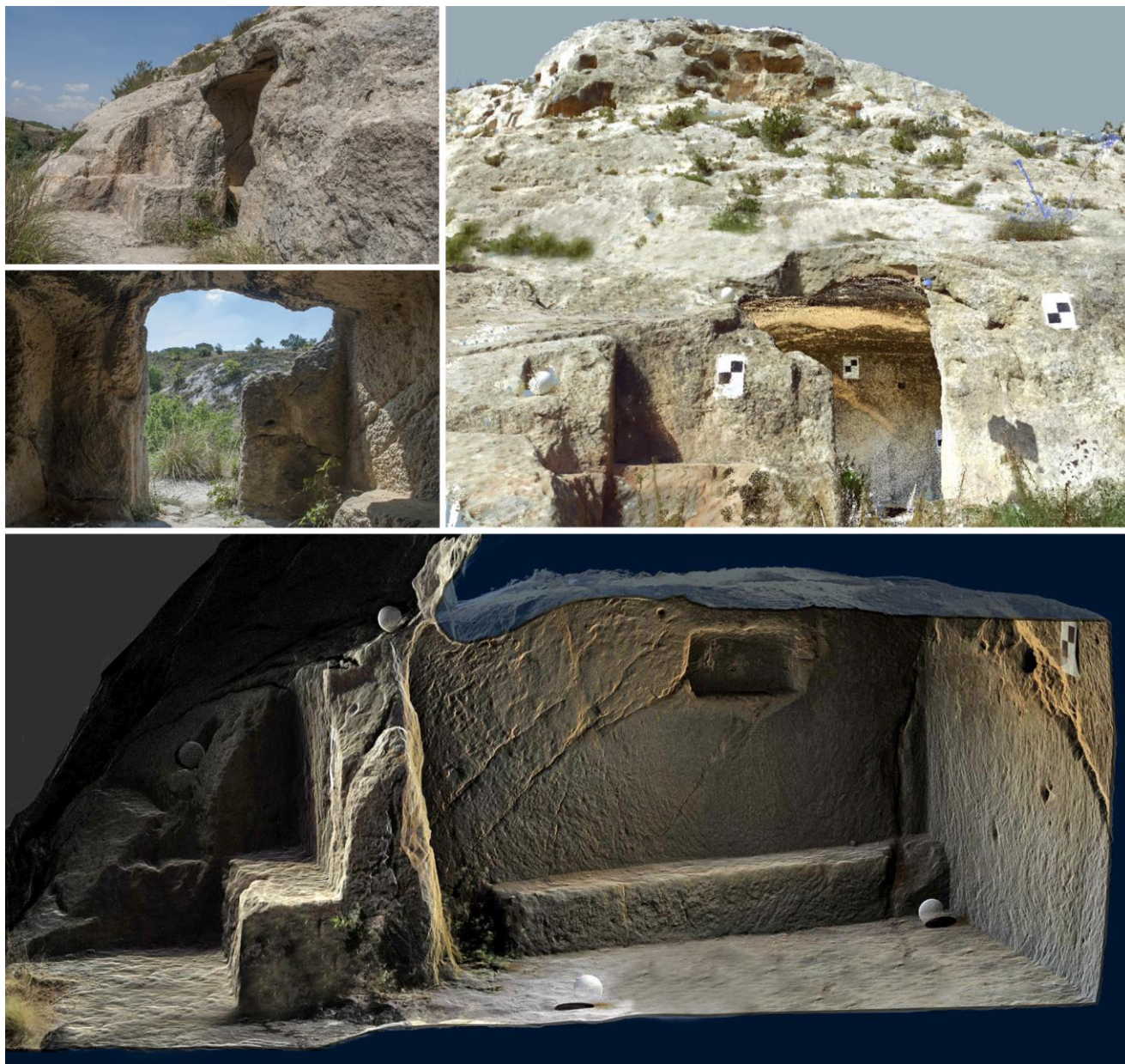
Fig. 9: The Necropolis of Realmese in Calascibetta - (from top to bottom) analysis of F20 tomb by 3D laser scanning, phases of the survey and the reconstruction of the longitudinal section from the point cloud.
