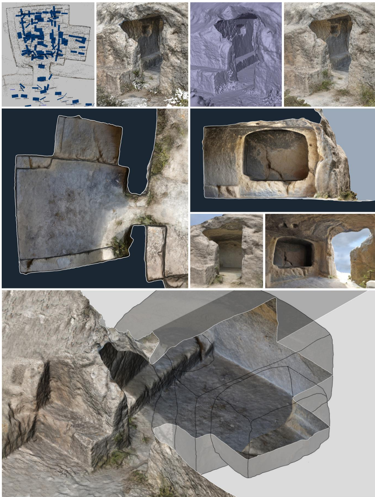
Fig. 8: The Necropolis of Realmese in Calascibetta - analysis of the F20 tomb. Example of image-based 3D reconstruction (top), floor plan, sections and views of the 3D model (center) and isometric view (bottom).
