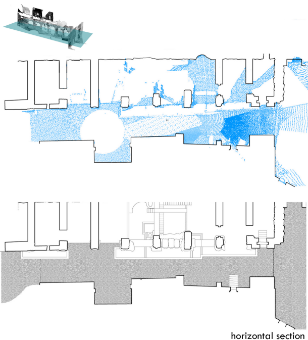
Fig. 10: From point cloud to 2D models. Horizontal section proportional interpretations of the whole complex.
