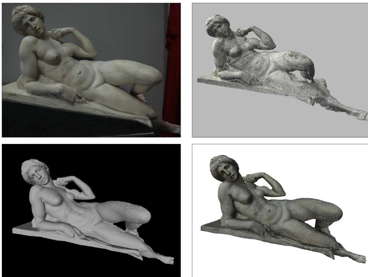
Fig. 1: Digital survey of the Michelangelo plaster works of the Fine Arts Academy of Perugia, 2015, Dawn : photographic view, point cloud, mesh, textured mesh
