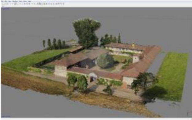
Fig. 13: Point cloud obtained by automated photogrammetric process on the drone captured images, Comollo (2016)
