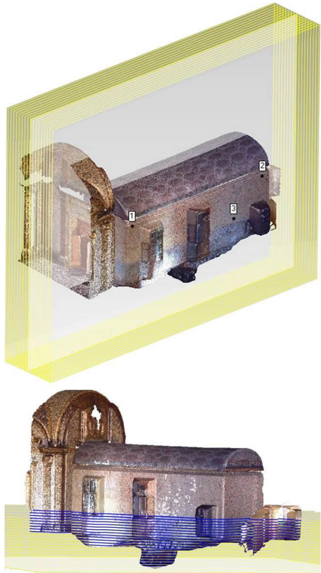
Fig. 8: Mesh model sliced from vertical and horizontal planes
