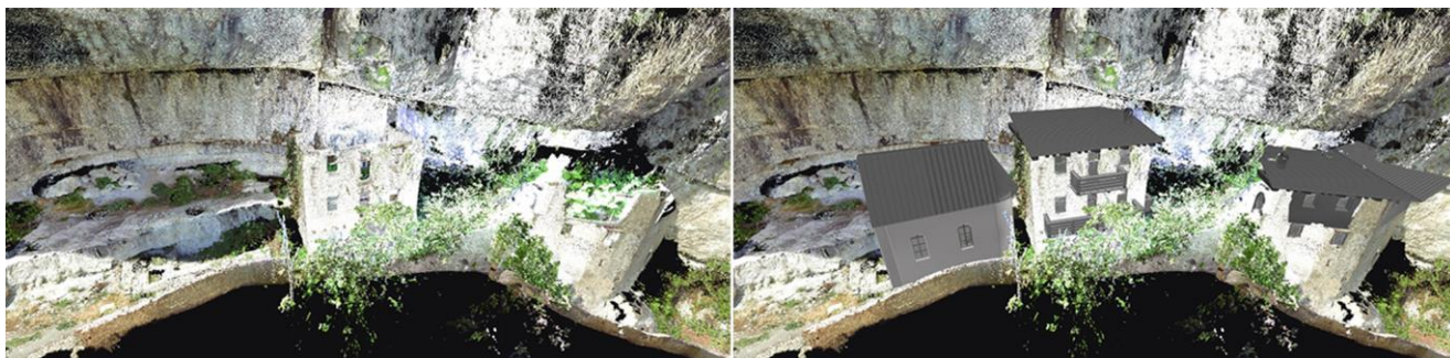
Fig. 14: A view of the 3D model before and after entering the volumes as they were, digitally rebuilt on the basis of historical and archival assumptions.
