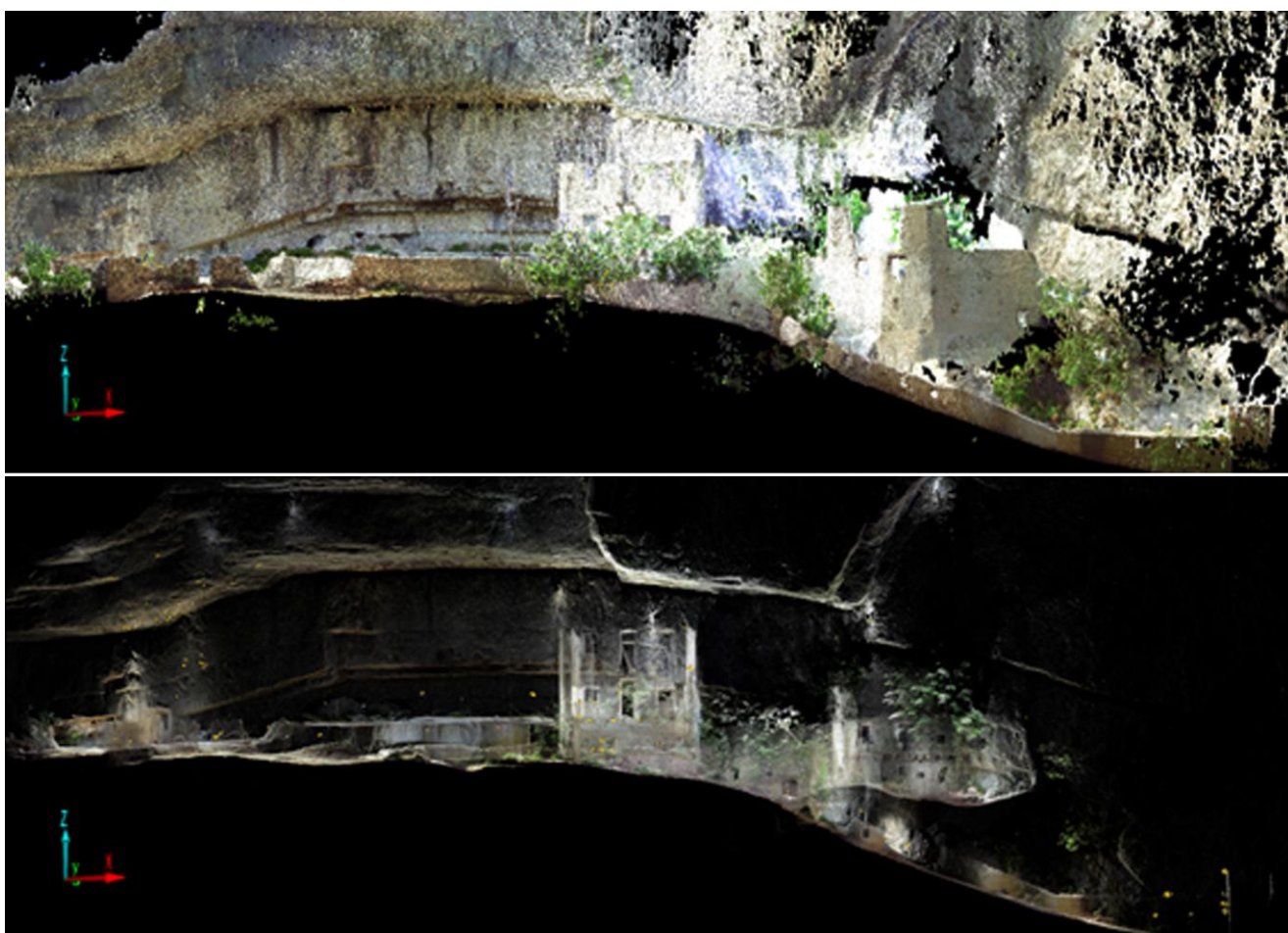
Fig. 8: 3D view of the “points cloud” finished recording; normal mode (top) and clear view mode (down).
