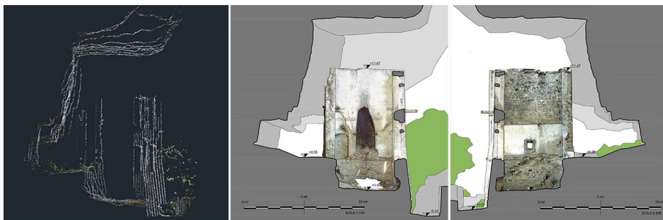
Fig. 9: The hermitage: graphic representation of the vertical east and west sections, coded for 1:100 print.
