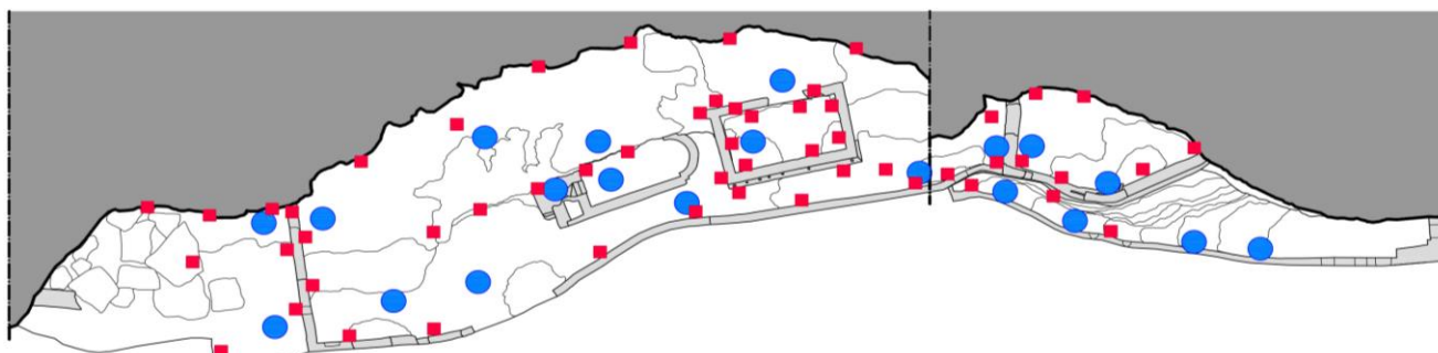
Fig. 6: The project of laser scanner survey and the view of a single scan: the instrumental positions are blue, the orientation targets are red.
