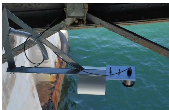
Fig. 5: Ultrasonic tide gauge installed in Mar Piccolo, South Italy (Source: De Serio & Mossa, 2016b).
