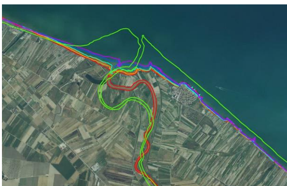
Fig. 1: Shoreline evolution of the Ofanto river (Apulia Region): 1943 (green line), 2005 (purple line), 2008 (blue line), 2013 (red line). (Source: Mossa, Nobile, & Petrillo, 2016).
