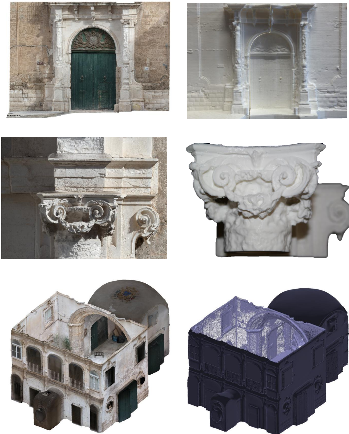
Fig. 2: Polygonal meshes (with textures) of the portal, the right ionic capital, and the internal atrium and courtyard; 3D printed models of the same elements
