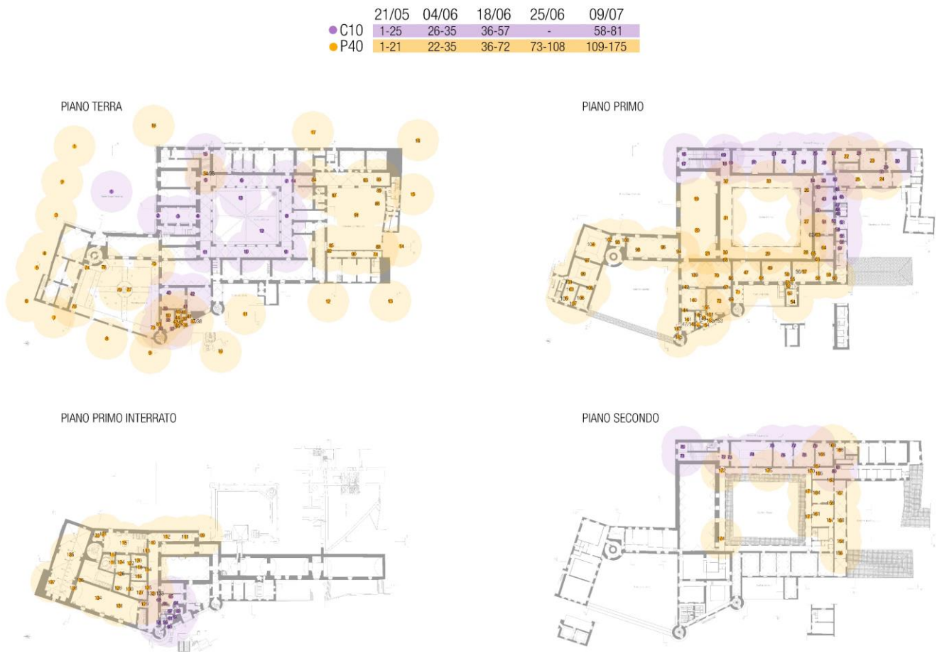
Fig. 6: Laser scanning survey: plans with scanner location. Two different tools used.
