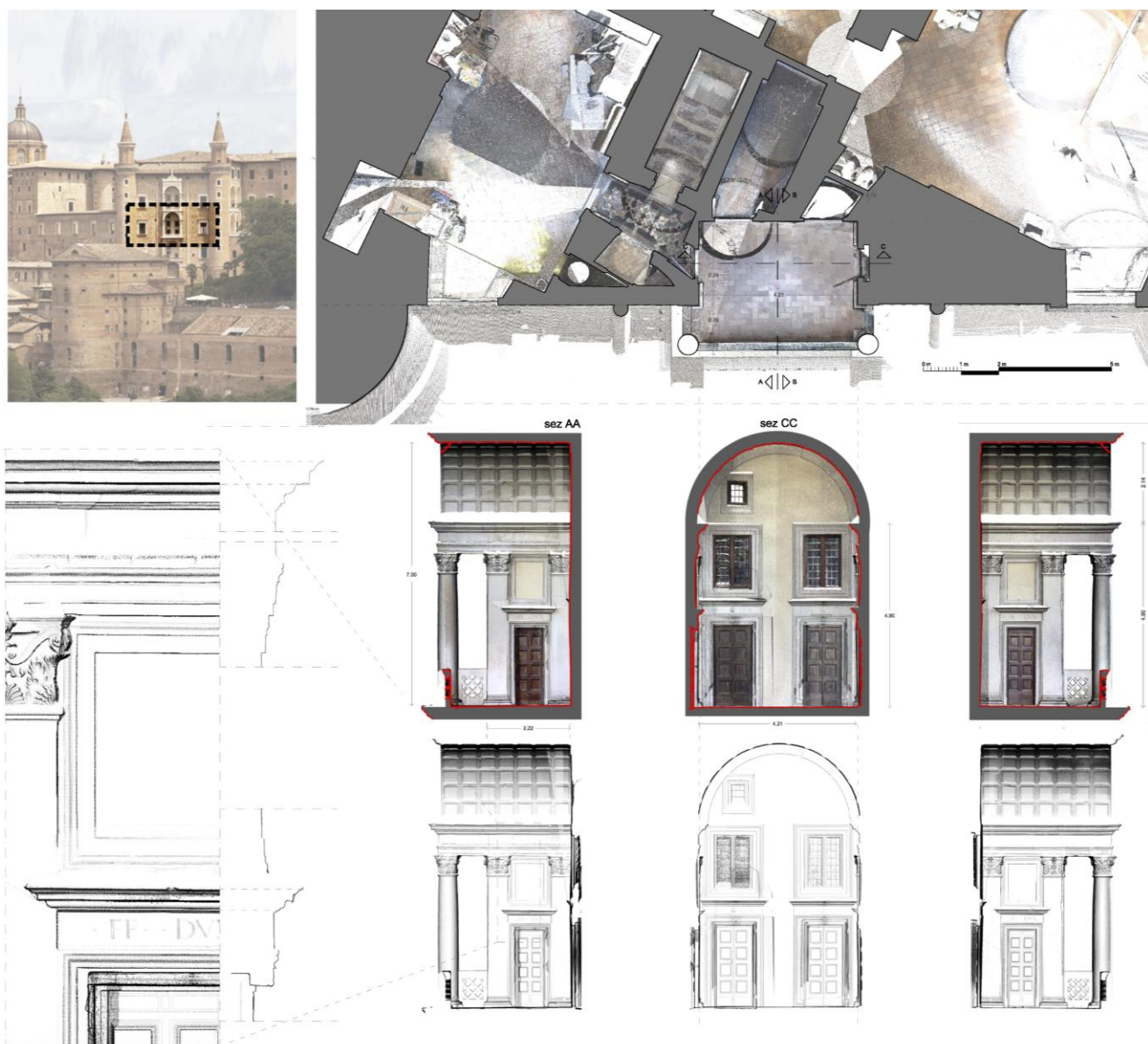
Fig. 9: Plan, sections and details of Loggia near the chapel of the Forgiveness and the temple dedicated to the Muses.
