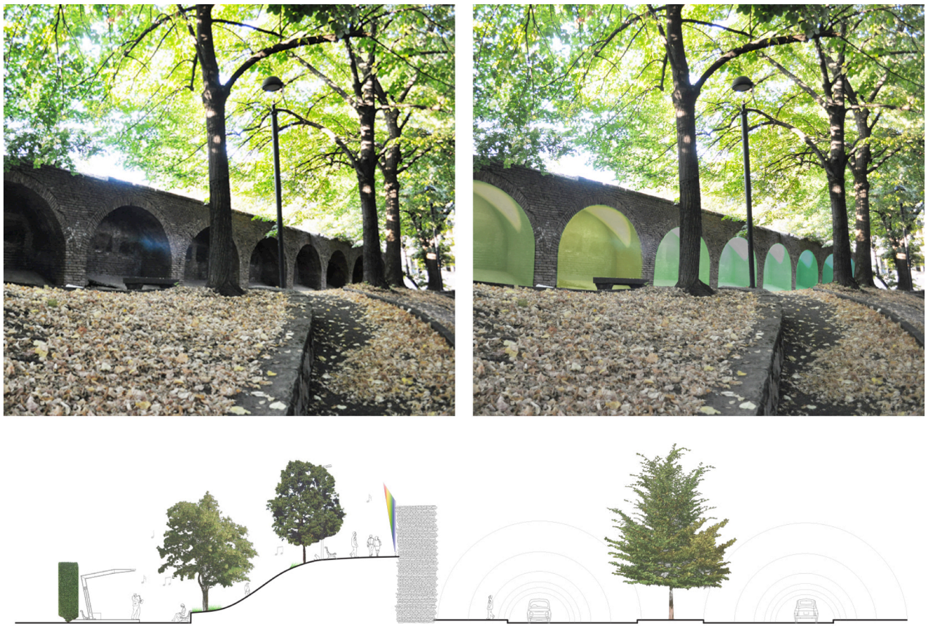
Fig. 3: Design graphic arts of the renewal intervention of Project Area: (top, on the left) photograph of the existing brick arcades delimiting the zone; (top, on the right) image representing the final suggestive aspect of the ancient walls coloured by the interactive installation proposed; (down) section representing the final design state.
