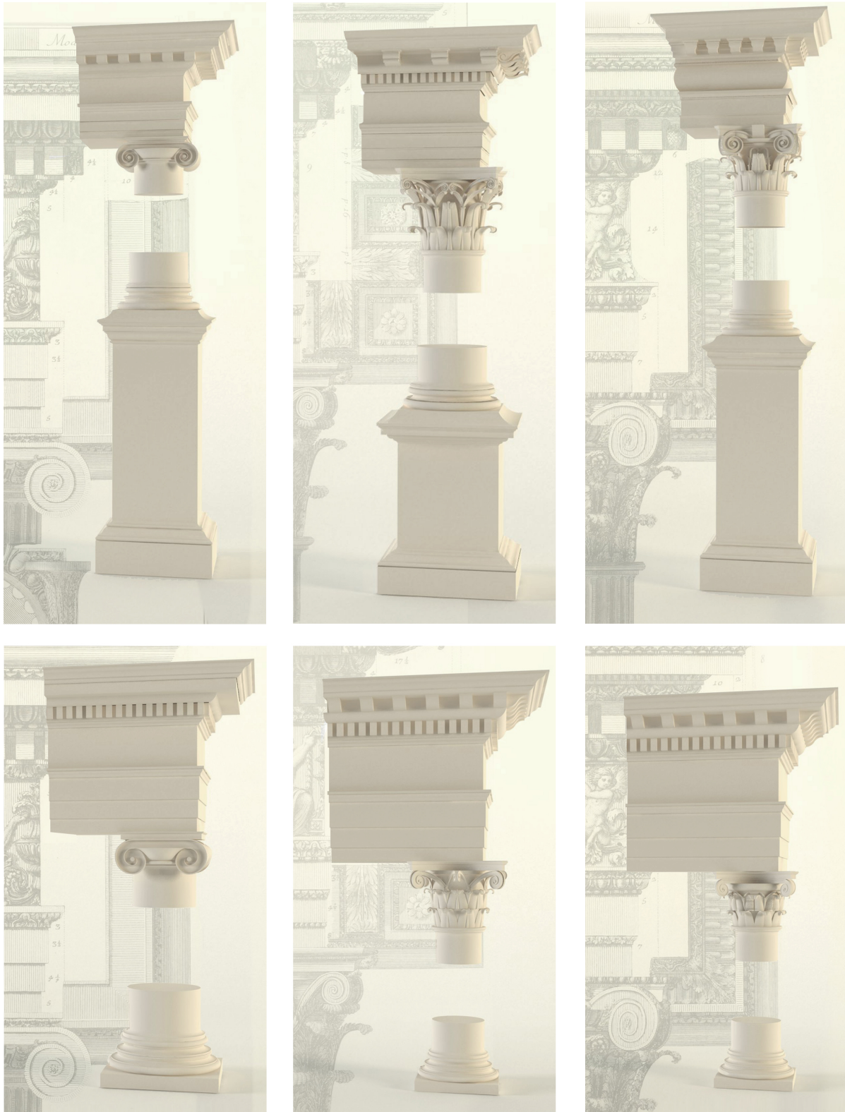
Fig. 10: Comparison between Palladio's (top) and Alberti's (bottom) Ionic, Corinth and Composite Order
