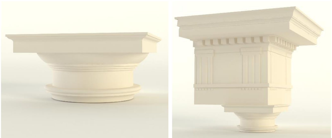
Fig. 3: Representation of the Doric capital and of its integration in the trabeation according to the Vignola interpretation
