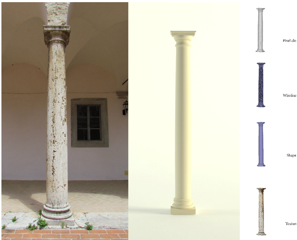
Fig. 13: Modelling of an existing historical the columns of St. Peter's Stars Courtyard in Perugia, designed by the architect Galeazzo Alessi
