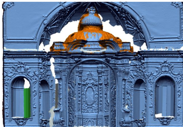
Fig. 6: Data integration of the laser scanner (blue): with photogrammetry (orange) and through extrusion of 2D reference (green)
