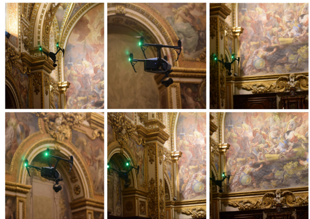
Fig. 16: Acquisition operations inside the sacristy of san Paolo Maggiore with drone and camera with 5K resolution.
