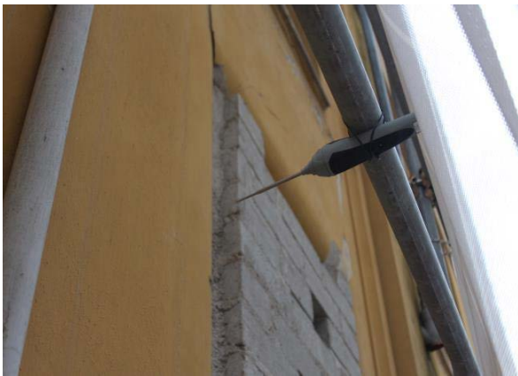
Fig. 17: The thermofluximeter probe, external view
