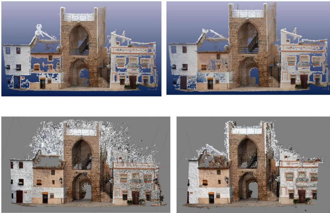
Fig. 9: Stereo point clouds obtained with Medium / High settings in PM (top) and PS (bottom), respectively, without pre-DSM filtering. It can be seen how a greater demand in the SFD + Matching and SGM / MVS algorithms, generally produces denser models, with a more uniform distribution of points and fewer clusters of outliers. This ensures a more precise metric evaluation, and a more sharp and uniform posterior mesh. Note: the displayed models are incomplete because the aerial photos are missing
