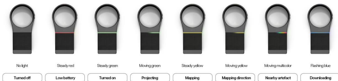
Fig. 7: The different configurations of Aura: each combination of colour and light movement corresponds to a specific state of action of the device
