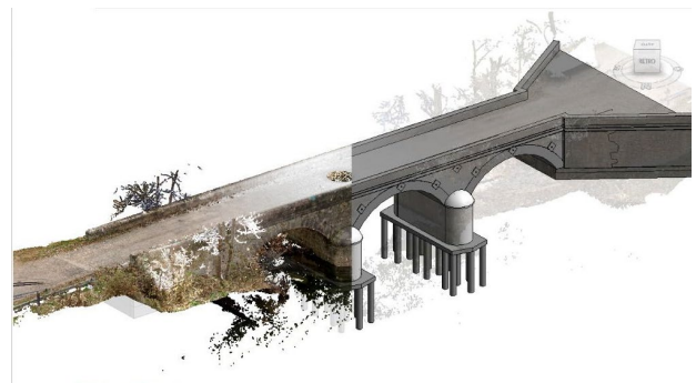
Fig. 4: Point cloud imported into BIM environment for the development of the parametric model of the bridge
