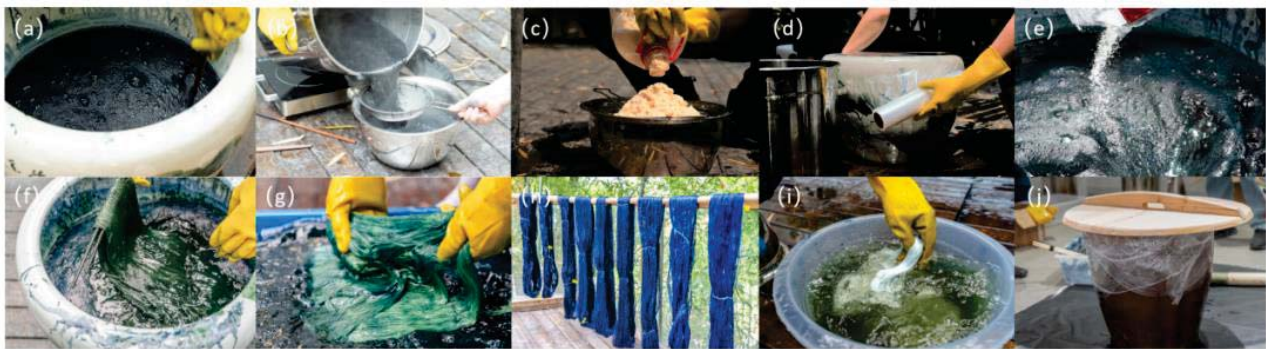
Fig. 5: The image record of indigo dyeing by the professional dyer Jisheng Wang: (a) Dissolve indigo mud in the vat. (b) Add alkaline straw ash filtrate to the indigo solution. (c) Add sweet fermented-rice filtrate to aid fermentation. (d) Seal the vat to create a suitable environment for fermentation. (e) Check the condition of the dye solution after several days. (f) Dip silk yarns in the vat for dyeing. (g) Rinse the silk with water. (h) Hanging the silk to reveal the blue colour by oxidation. (i) Dye other silk yarns for different time or in different concentration. (j) Add some materials, reseal the vat, and continue fermentation for the next dyeing.
