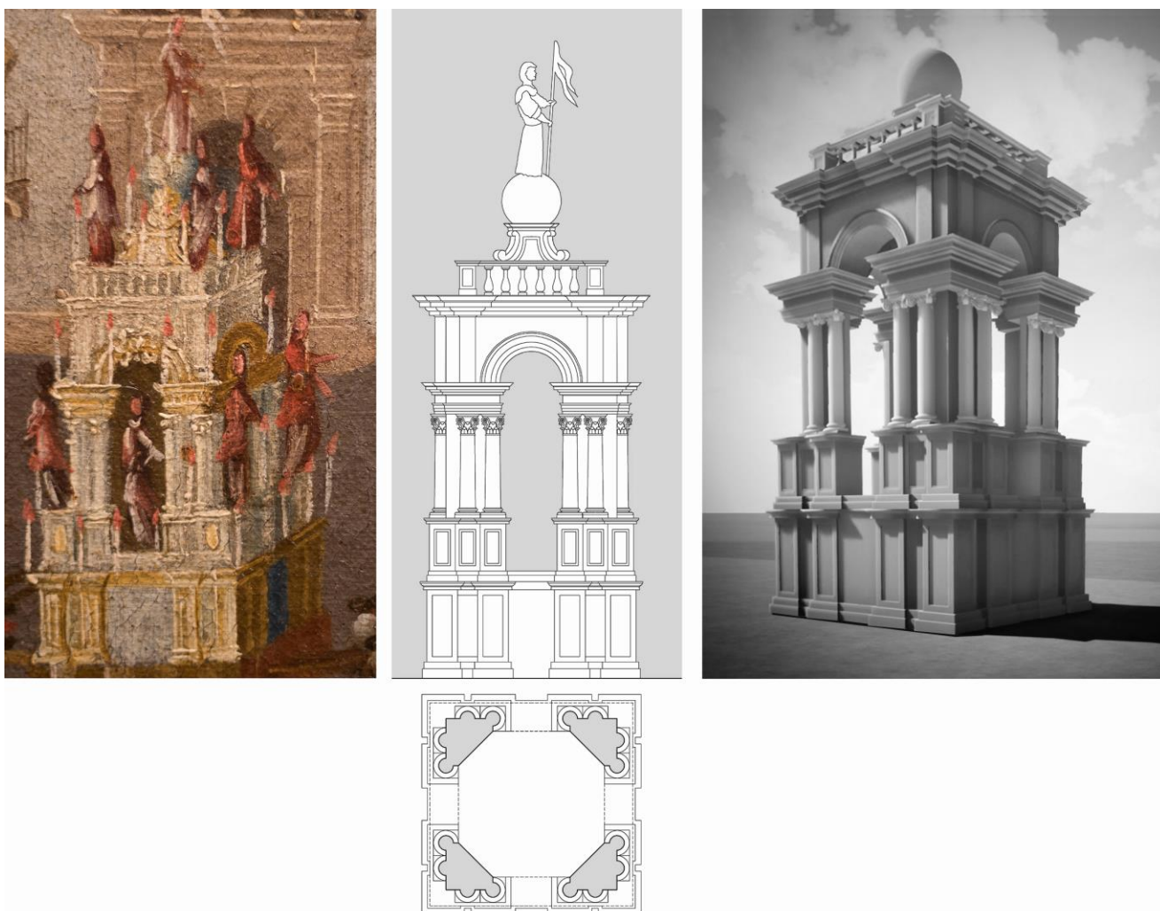
Fig. 8: Excerpt from The Procession painting, reconstruction in plan and elevation, and rendering from the 3D solid model of the last ephemeral machine of the procession (Drawing by F. Colonnese; rendering by L. Ascani).
