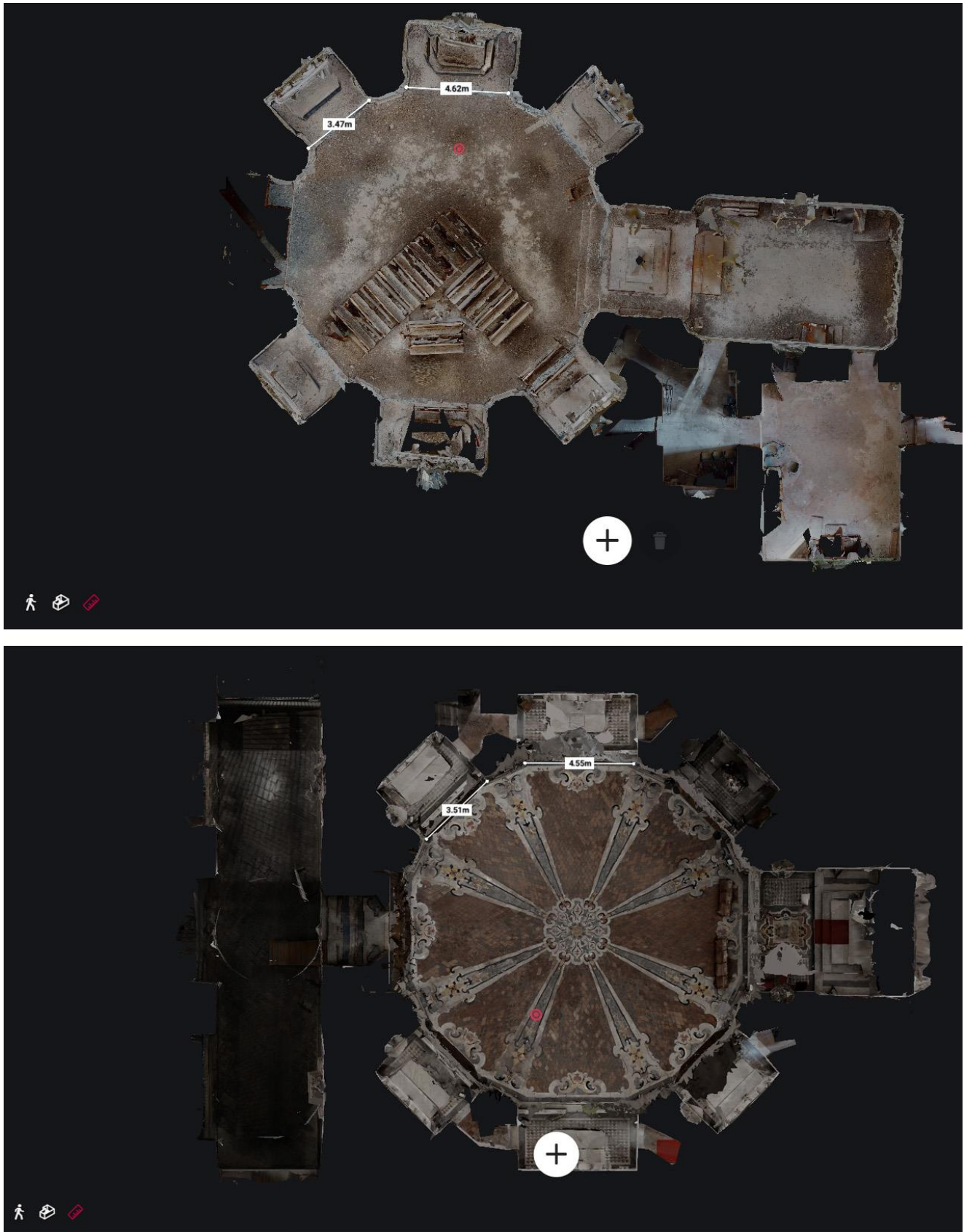
Fig. 12: Navigable model of the Church of Santa Maria della Purità (upper image) and the Chapel of Pio Monte della Misericordia (lower image). Comparison between the two buildings is facilitated by the possibility of taking measurements.
