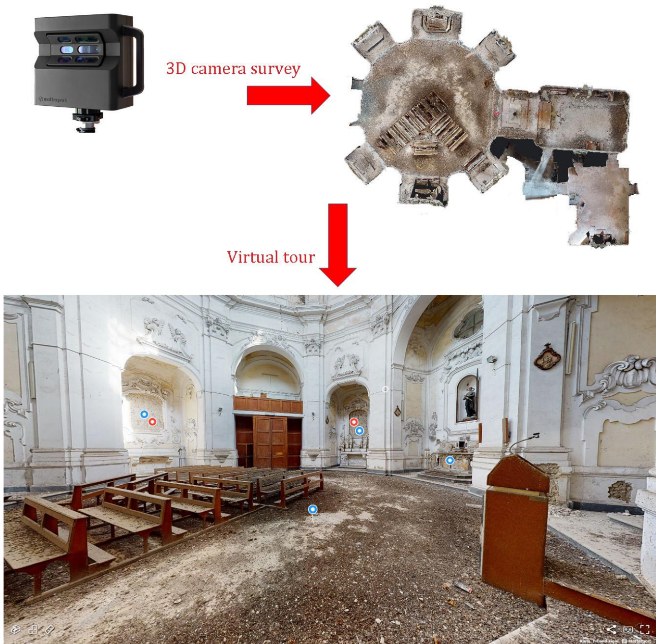
Fig. 6: Survey workflow. From the 3D camera survey to the virtual tour. Survey by Mario Ronca, supervisor Manuela Piscitelli.
