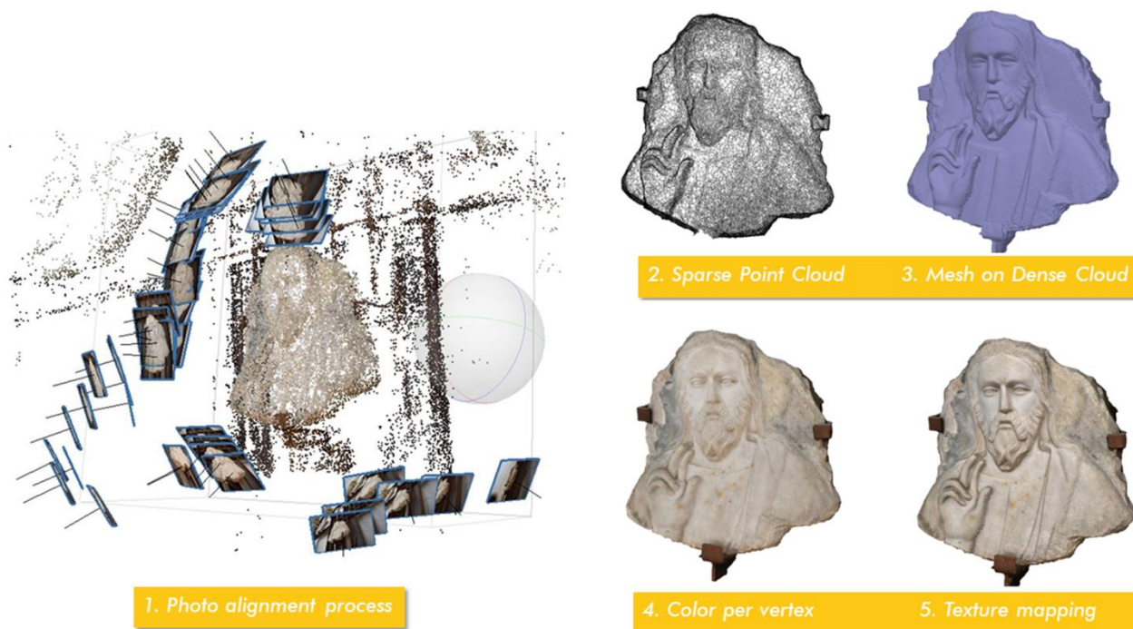
Fig. 3: Phases of the photogrammetric process applied to the case study of medieval sculptural pieces. The example of the Blessing Christ (author's image)
