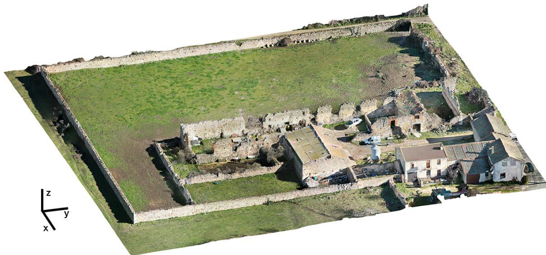
Fig. 6: Axonometric view of the photogrammetric survey model. By the author.
