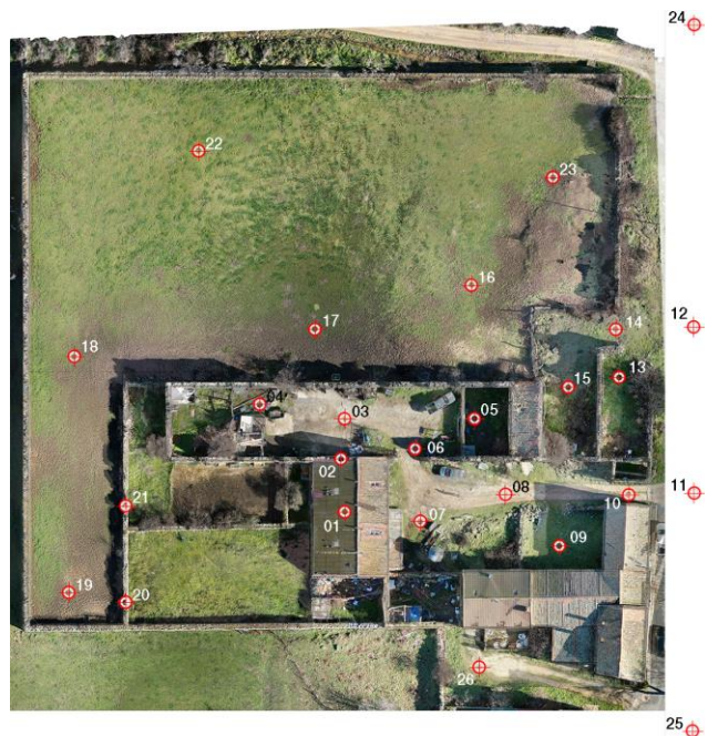
Fig. 7: Location of scanning stations. Combined plan of scanner and photogrammetry models. By the author.
