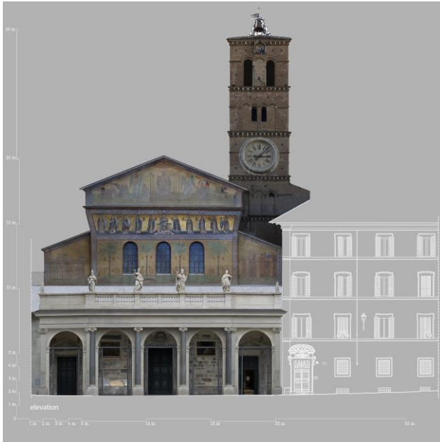
Fig. 8: Orthoimages of the main facade
