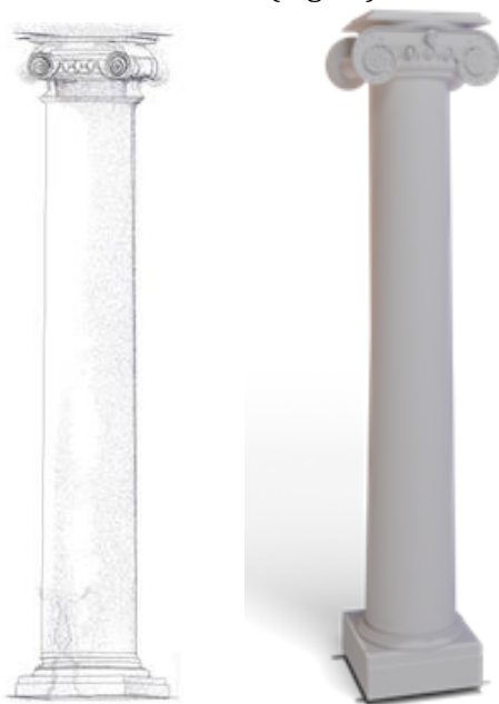
Fig. 11: Point cloud inside the family around the model with the adaptive point component and example of one modelled architectural order
