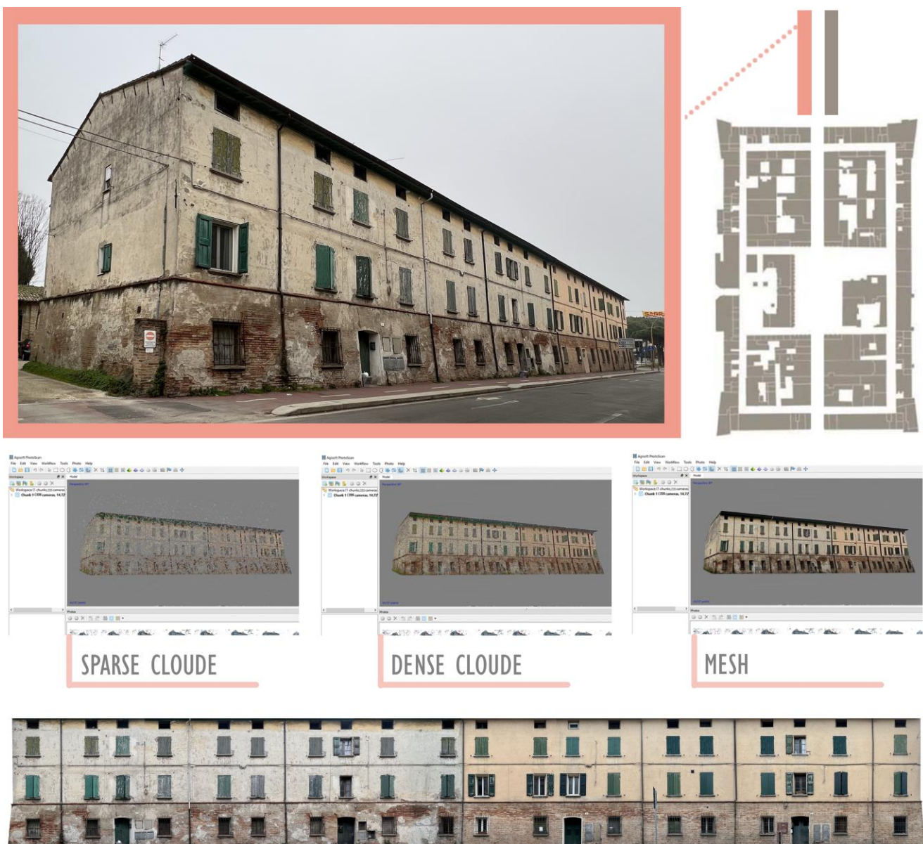
Fig. 5: Image processing in Agisoft Metashape software of the complex in Borgo Saffi and orthophoto derived from the model (elaboration by authors).
