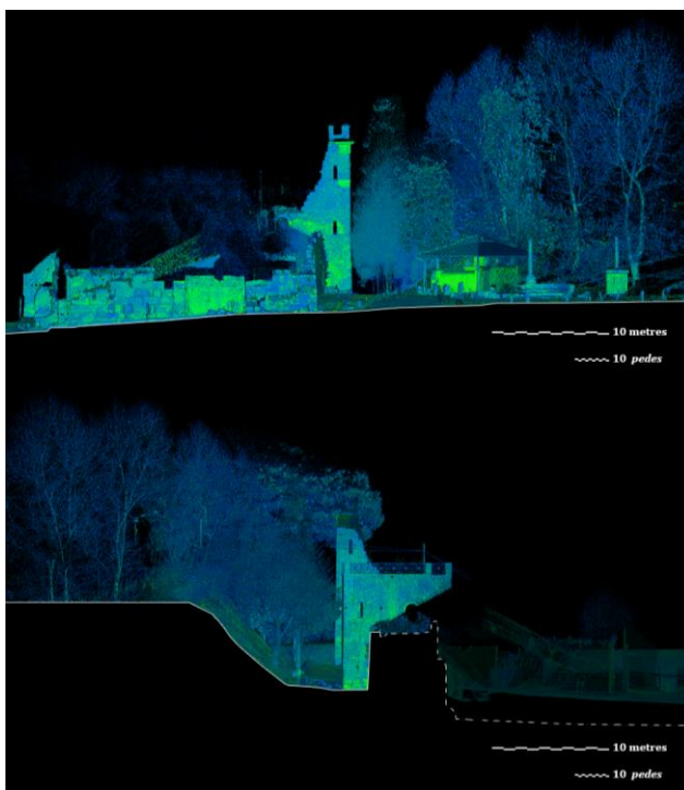
Fig. 7: Two views of the TLS point cloud: on the top section along the street of Vesuvio Gate; on the bottom section on the western side of tower XI. Credits: S. Bertacchi
