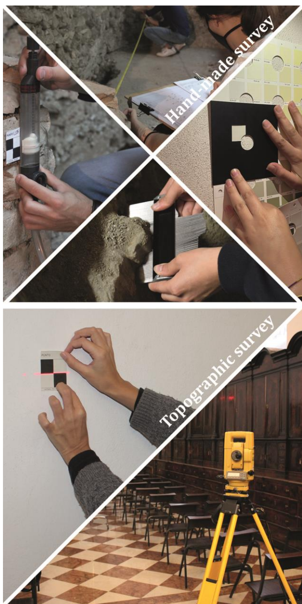
Fig. 2: The traditional methods used for acquiring the geometric and colourimetric data of Pretorio Palace; from top to bottom: hand-made survey and topographic survey.
