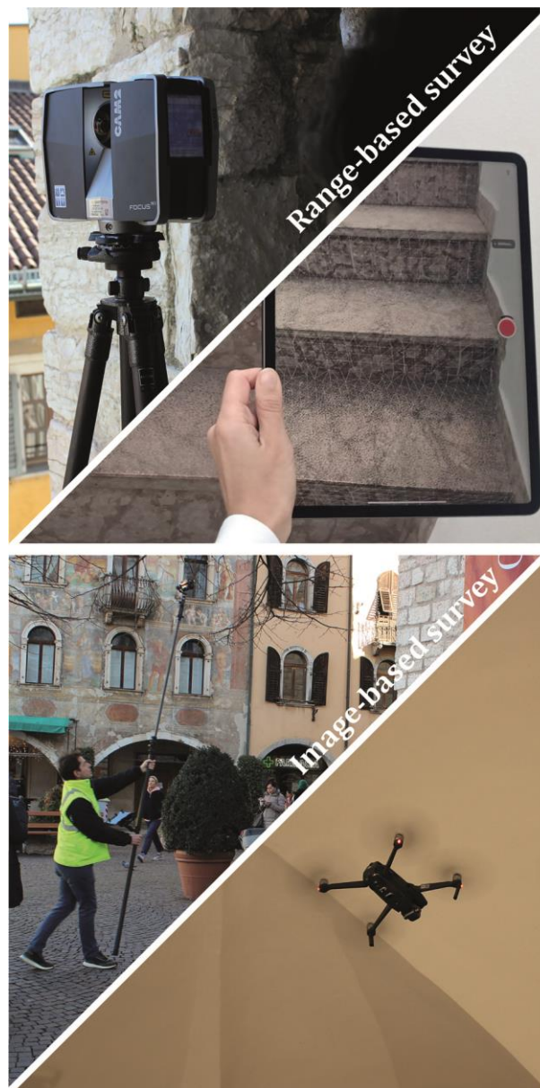
Fig. 3: The digital methods used for acquiring the geometric and colourimetric data of Pretorio Palace; from top to bottom: range-based survey (i.e. Terrestrial Laser Scanner, tablet with LIDAR sensor) and image-based survey (i.e. terrestrial and aerial cameras).
