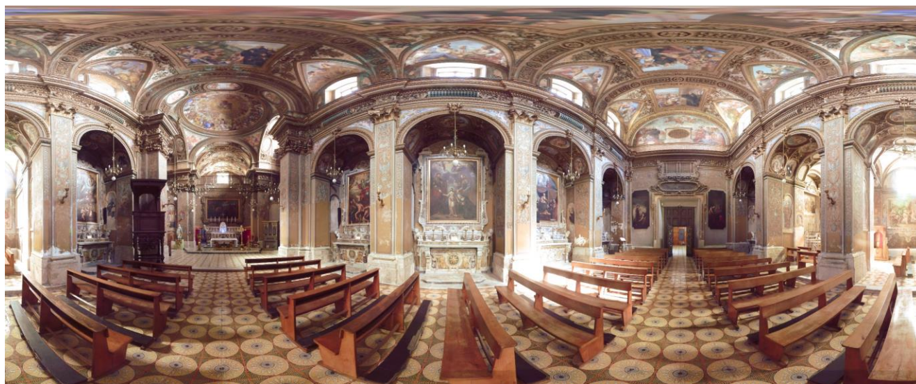
Fig. 11: Equirectangular projection of a 360-degree photographic acquisition used as input for the body of the Virtual Tour.
