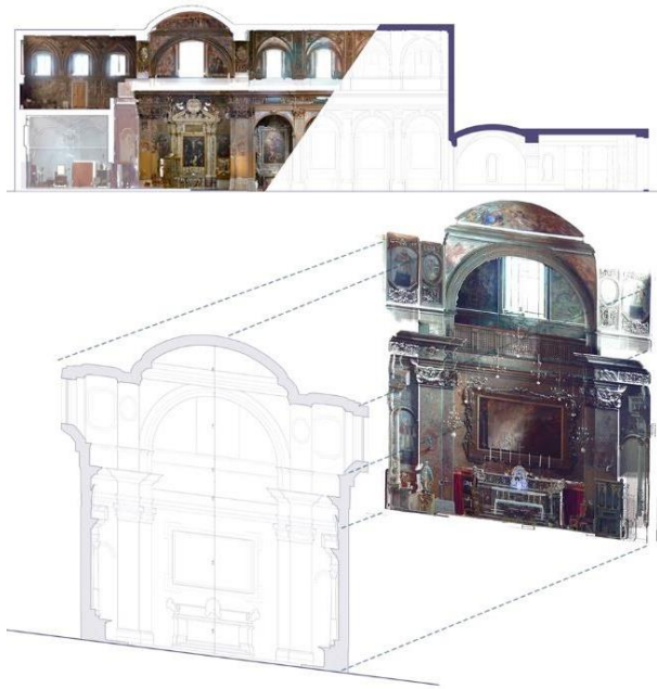
Fig. 8: Vectorisation of orthophotos produced by close-range photogrammetry.
