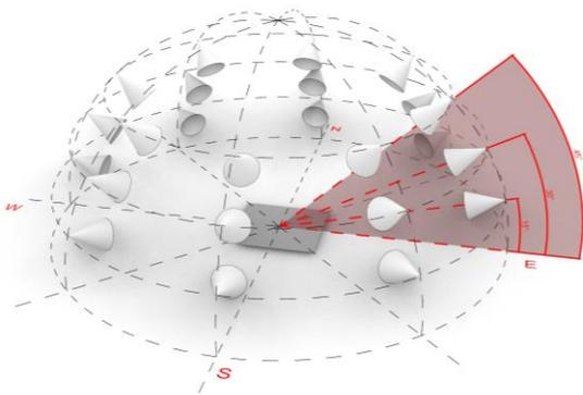
**Fig. 5:** The suggested light layout around the sample
