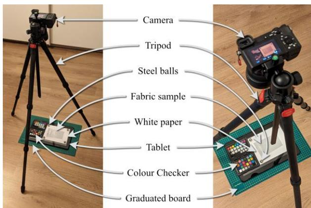
Fig. 3: Fabric acquisition setup
