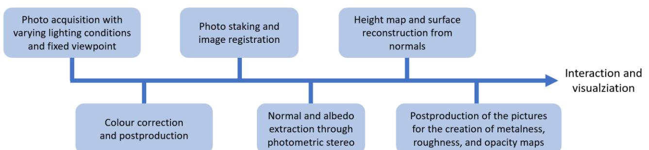
Fig. 2: Low-cost digitization workflow of samples of fabrics
