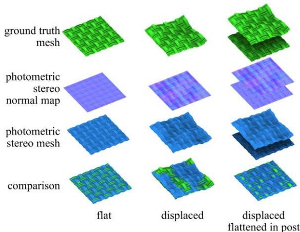
Fig. 9: Comparison between ground truth 3D models and output geometry acquired through photometric stereo.
