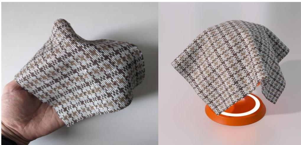
**Fig. 7:** Textured woven fabric sample test. Left real sample, right simulated sample (Blender cycles)
