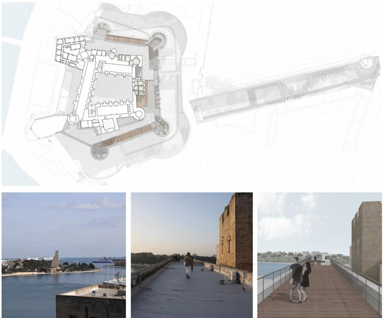
Fig. 13: The Great Castle of Brindisi. Overall plan +12,5 m, foreshadowing of the possible design outcome (a), panorama visible from terraces (b), the terraces at roof level, current state (c) and foreshadowing of the possible design outcome (d) (photos and graphic elaborations by Chiarello G., Ferrante A., Lamorgese R., Liddo G., Strippoli F., 2022)
