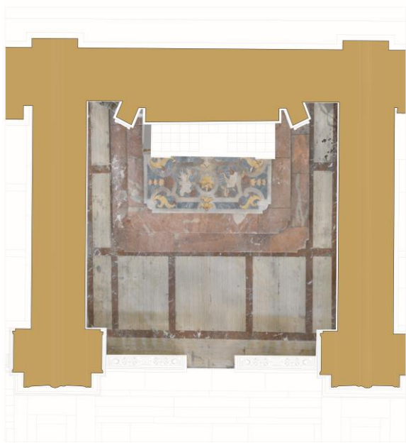
Fig. 5: Photogrammetric survey of the flooring of the Chapel of the Holy Rosary in St. Catherine's Church (elaboration by student architect M.R. Campo, a. y. 2022-23)
