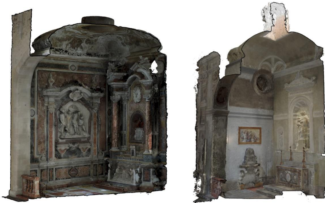
Fig. 2: Structure for motion models of the Hecce Homo and Madonna degli Angeli chapels, located in the right aisle of the Church of St Francis of Assisi. 2023 (graphic elaboration by the students of the "Laboratory of Monument Restoration", 2022-2023).
