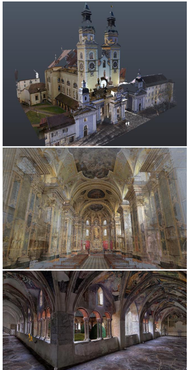
Fig. 5: B_Digital project: the survey of the Brixen cathedral (views extracted from the point cloud).
