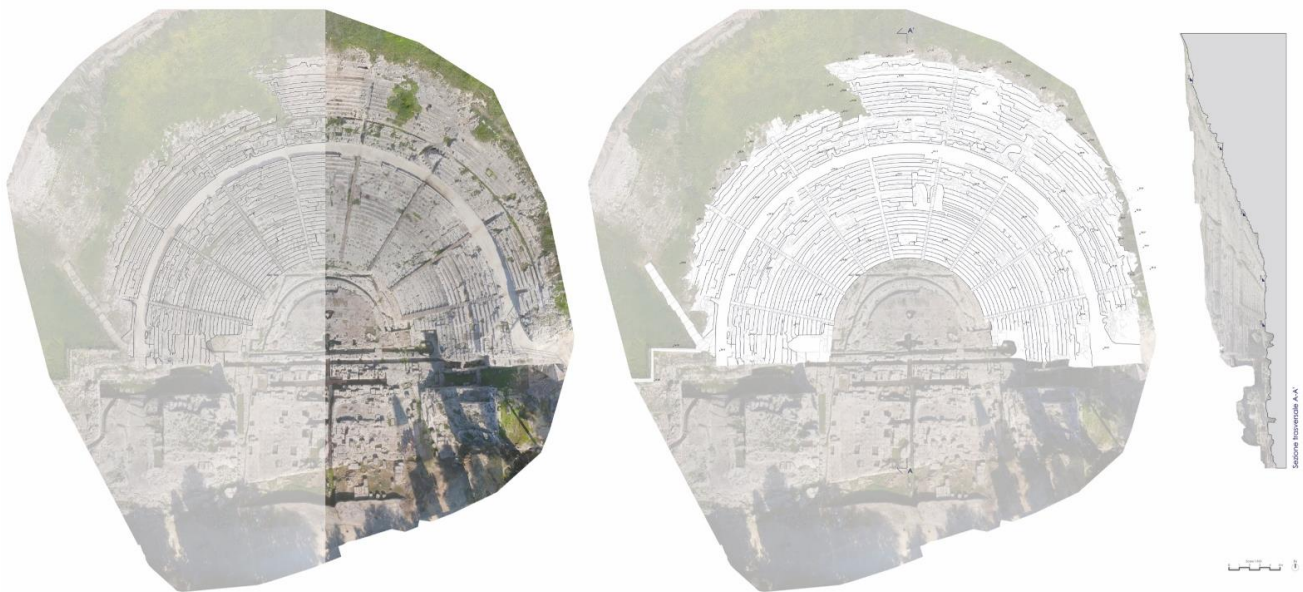
Fig. 4: Orthophotos and 2D representations of the survey
