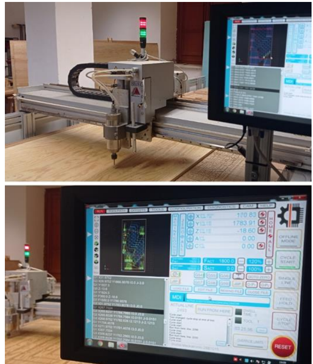
Fig. 8: LAMM laboratory: CNC milling of the prototype components system equipment's.
