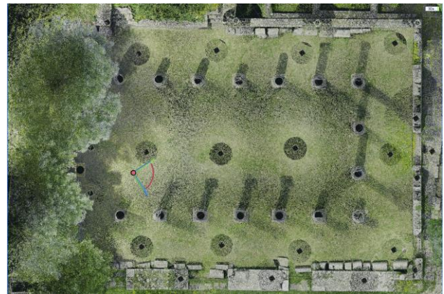
Fig. 7: Locating station points with the laser scanner in the survey phase by visualising quadrics in Reality Capture.
