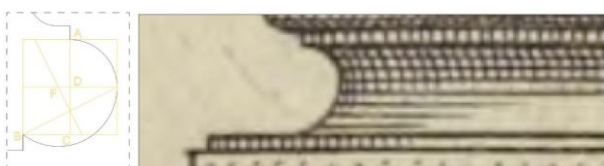
Fig. 5: Geometric construction of the Scotia.
