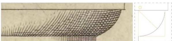
Fig. 4: Geometric construction of the Ovolo.
