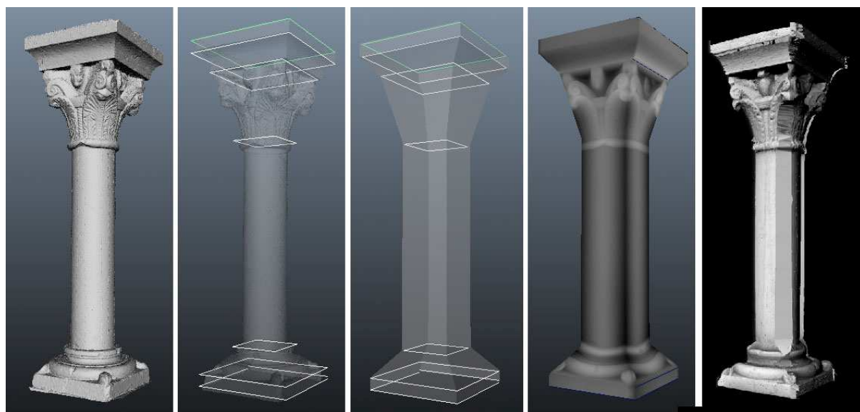
Fig. 5: Process of mapping visual information and geometry on geometric primitives through the creation of "enriched textures".
