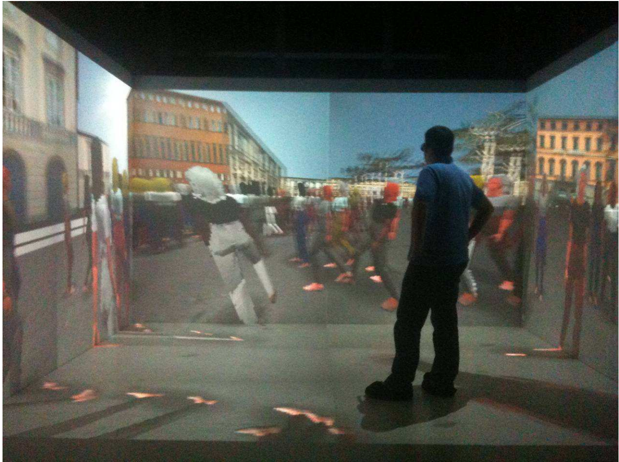
Fig. 6: Immersive Rendering of Crowds in the X-Cave at PERCRO laboratory
