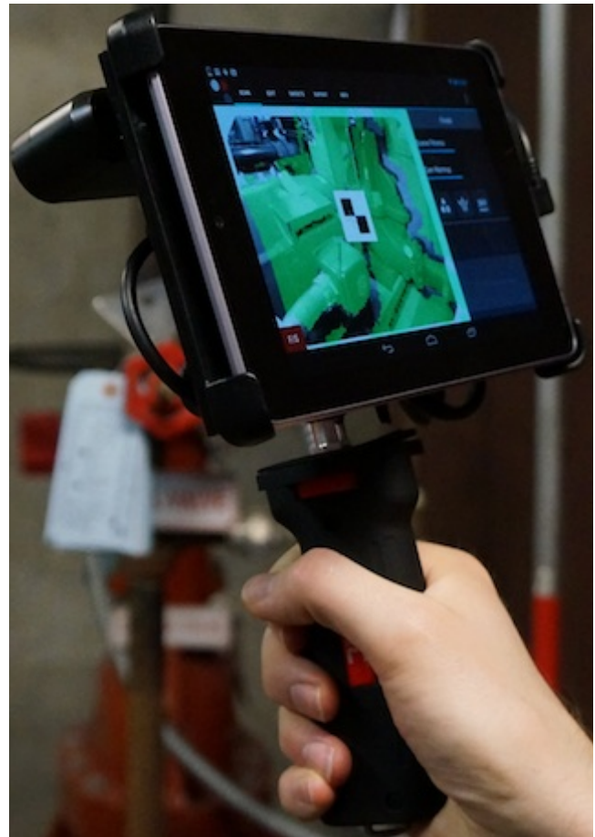
Fig. 6: Photogrammetry-based device for 3D capturing
