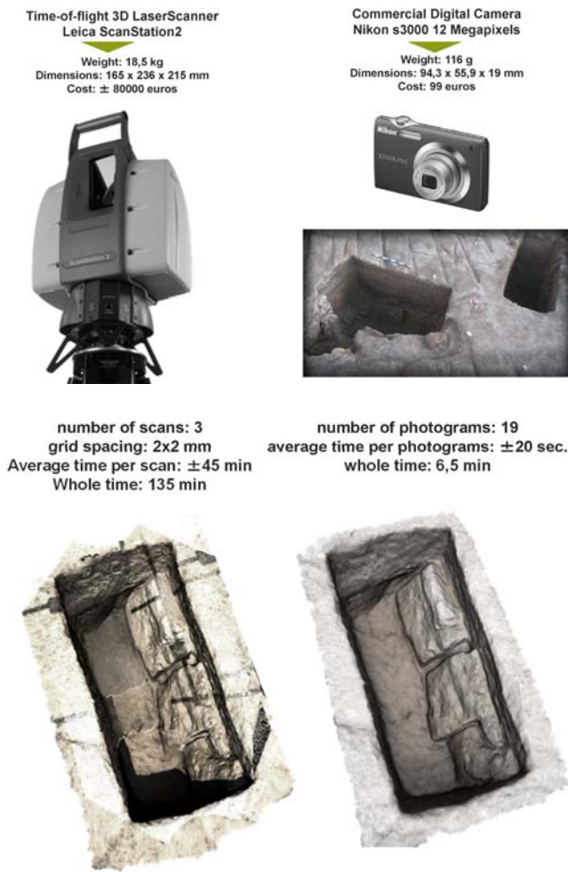
Fig. 5: 3D scanning vs. Image Based Modelling: a cost/benefits comparison (Crustumarium tombs survey - Rome)
