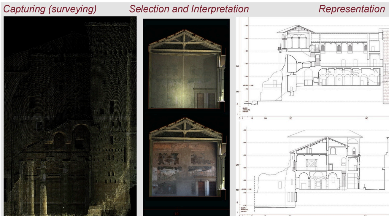
Fig. 1: The three phases of the Survey process : Data capturing, Selection/Interpretation and Representation (Casa dei Cavalieri di Rodi – Rome)
